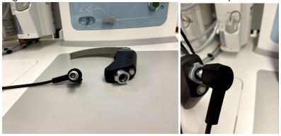
3) Plug in the connector into the C-Mac blade and the blue light on the handle as well as the main light on the blade should automatically turn on.
